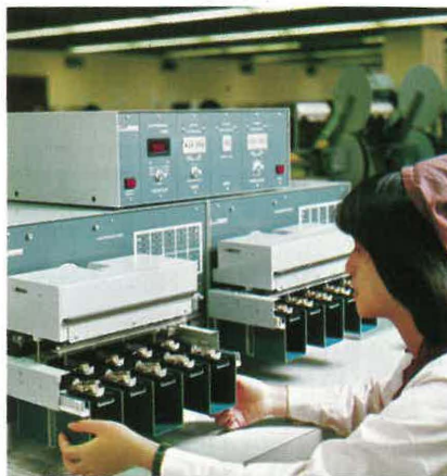
Stelux's watch manufacturing facilities are designed and equipped to international standards. These pictures show (from top) a sophisticated automatic system used in the electroplating of watch bands; the testing of completed watches; and the assembly of watch movements.
